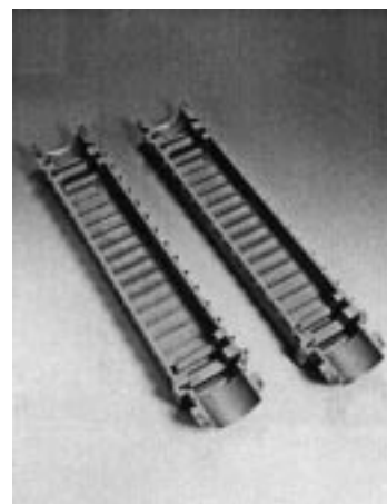
Fig. 10. Clam-shell mounting arrangement of the eight-iris polarizer (top) realized with a square waveguide including two square-to-circular (26-mm diameter) transitions. As an example of clam-shell mounting arrangement (bottom), an open polarizer working in S -band is shown. The clam-shell mounting consists of manufacturing two identical symmetrical halves, which are then joined together.
